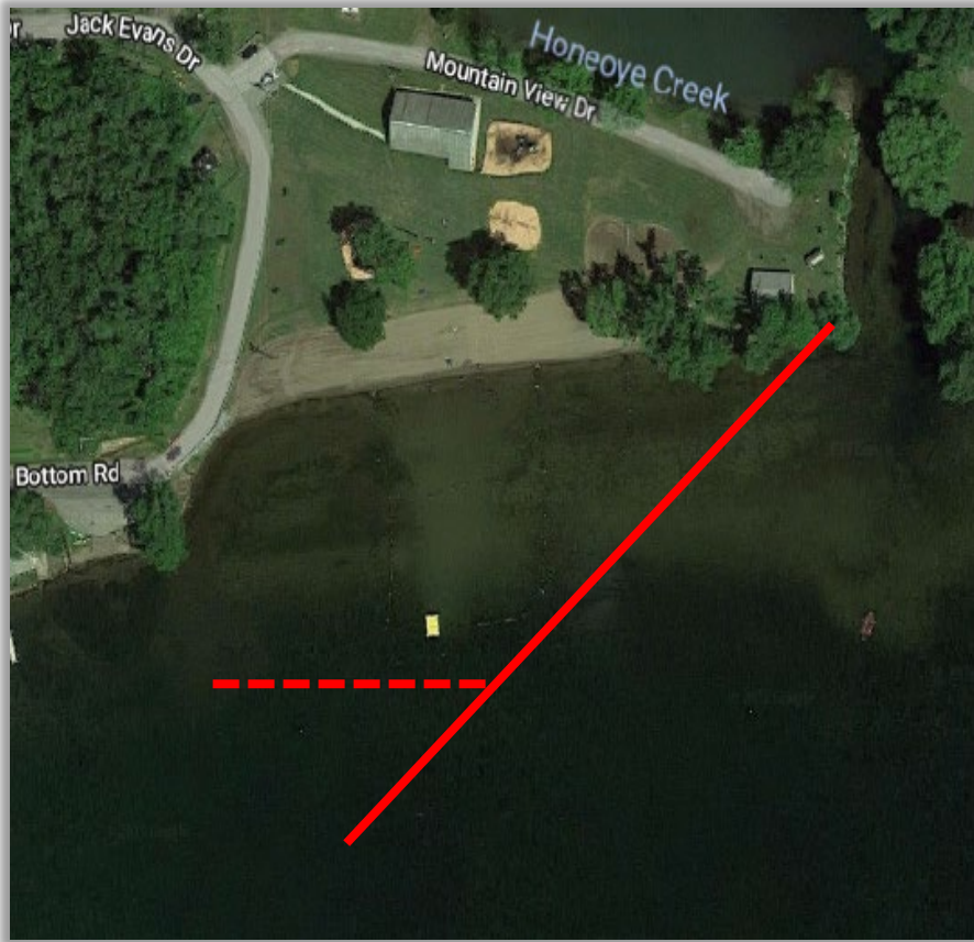
Figure 5.2 Sedimentation Curtain Installation Options
